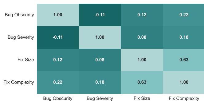
(b) Correlation matrix illustrating relationships between ordinal study factors. The data shows a slight negative correlation between bug severity and obscurity ( -0.11 ), and a minimal correlation between bug severity and fix size ( 0.08 ), suggesting that the potential impact of tooling for detecting/fixing shallow bugs should not be discounted.
